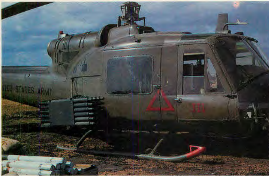
ABOVE: B-model Aerial Rocket Artillery (ARA) gunship, or "hog," carrying 48 2.75-inch HE rockets, which may be fired in any combination or all at once. Note 2.75-inch rockets at rearming stations on either side of ship with protective metal covers on rear over fins and electrical contacts. LEFT: Warrant Officer Sisk holds shrapnel from blown ammo dump, collected from area around his tent. Note Air Force-type survival knife and .45 automatic worn by flight crews.
